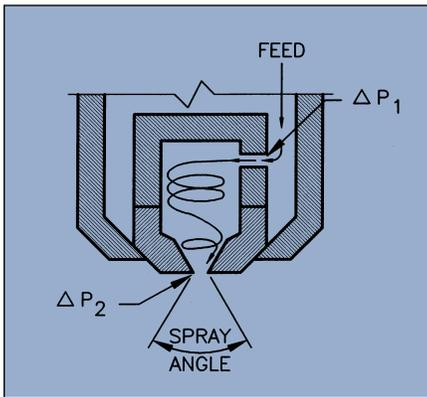
Figure 1: An example of a pressure nozzle
