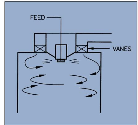
Figure 8: Cyclonic flow (fast mixing)
