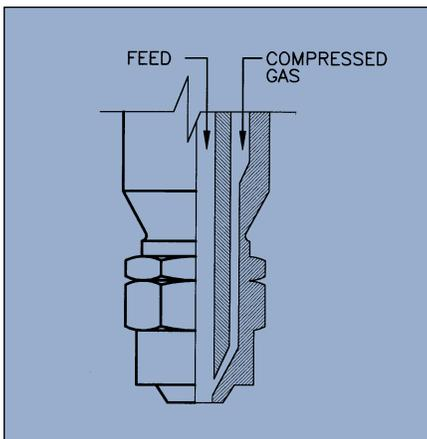
Figure 2: An example of a two-fluid nozzle
