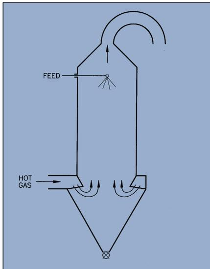
Figure 5: Counter-current flow
