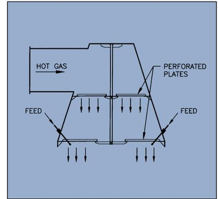
Figure 7: Parallel flow (slow mixing)
