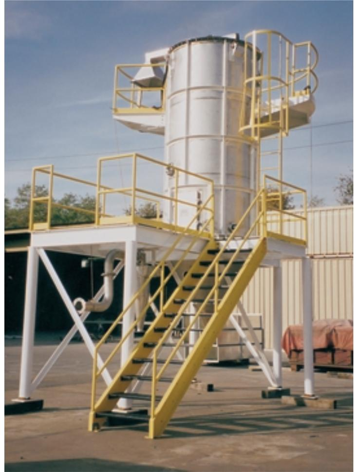
*This spray dryer was designed for a ceramic powder. It can be set up for co-current or mixed flow configuration.*
