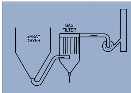
Figure 10: An example of single point bag filter collection
